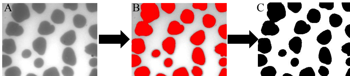
Figure 12: Example of ImageJ software analysis for determining the percent area light vs. dark. (A) the original image, with enhanced contrast. (B) The threshold selection for dark area is represented by the red coloring of the image. (C) Image J converts all areas that are not red into white, and the red areas into black to determine percent dark. This image shows a percent dark area, i.e. percent condensed domains, of 41.12%.
